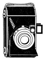
The  $2\frac{1}{4} \times 3\frac{1}{4}$  in. Nettar takes 8 exposures on standard 120 film. A brilliant reflecting view-finder is fitted as well as the direct vision finder. The f 7.7 lens is mounted in a two-speed shutter. Later models carry faster lenses and multiple speed shutters and are also fitted with a body release. Code No. 510/2.
