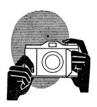
$2\frac{1}{4} \times 3\frac{1}{4}$  in. models: For upright pictures hold the camera with the right hand from above. The thumb of the left hand lies against the body release whilst the camera is supported from underneath by the palm of the left hand.
