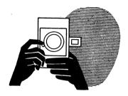
Early models without body release: Hold the camera against the nose with the right hand. Place the index finger of the left hand on the shutter release, and support the camera front with the palm of the left hand.
