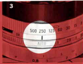
3. Set the aperture ring to AUTO mark.
