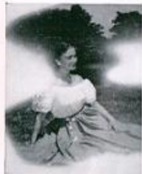
NEGATIVE ROLL LIGHT-STRUCK IN LOADING Note white streaks across picture. Do not break Scotch-Tape seal.
