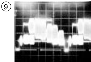
⑨ IC501 Pin ④⑤ 500mV/10μS EE/PB modes (V-OUT)
