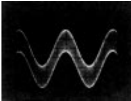
IC301 Pin ⑥ REC mode 2.2Vp-p
