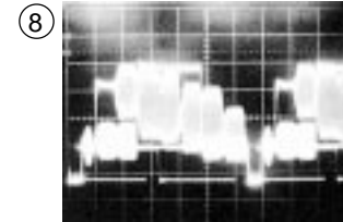
⑧ IC501 Pin ④③ 100mV/10μS EE/PB modes (V-IN)
