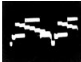
IC301 Pin ㉕ PB mode 400mVp-p
