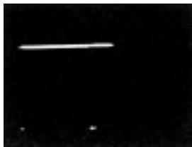
IC301 Pin ㉔ PB/REC mode 5Vp-p
